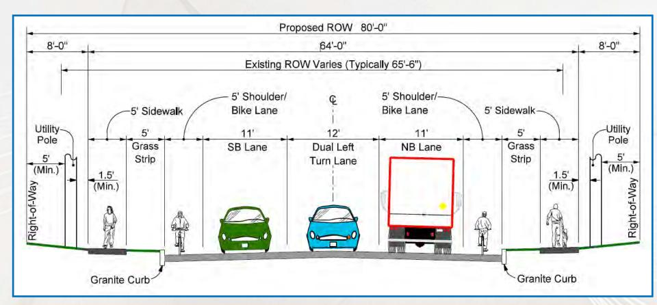
Typical Section – Three Lanes with Bike Lanes & Sidewalks on Both Sides (Willand Pond Road to Works Way – 2.0 mi)
